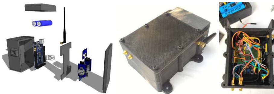
Figure 2. Housing (dimensions: 131 x 158 x 70 mm), external and internal components of WILD BIRD systems.
