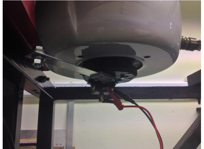
Figure 3. Cantilever energy harvester attached to permanent magnet shaker for provision of controlled base excitation
